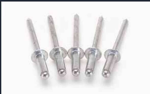
RIVET - ALUMINUM 3/16" X 4066804 [(.251)(.375)] DRILL #11
